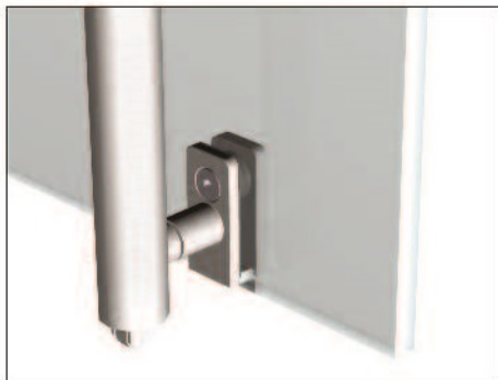
Glass Mount Detail at Latch
